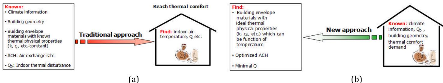
Figure 1 - Comparison of the traditional approach and the new approach for space heating and/or cooling: (a) traditional approach; (b) new approach;
