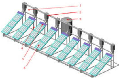
Figure 1- Universal solar water heating system (UniSheat) with rated productivity 1500 liters of water heated up to 90°C per day or 150 liter of steam at the temperature  $T \leq 120^\circ\text{C}$ , when solar insolation equals  $\approx 1000 \text{ W/m}^2\text{s}$ .
