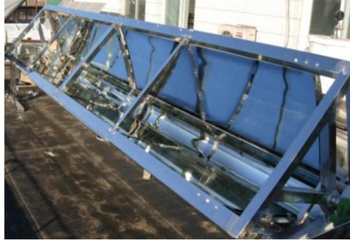
Fig. 1 The photo of the novel trough solar concentrator
